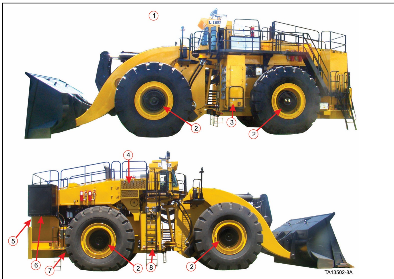
Figure 2: Special cleaning requirements (typical machine)
